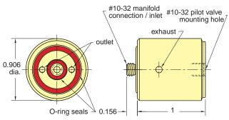
**Type:** 3-Way Normally Closed, Pressure Piloted Valve
