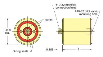
Type: 2-Way Normally Closed, Pressure Piloted Valve
